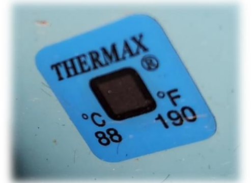
Overheated operating temperature
